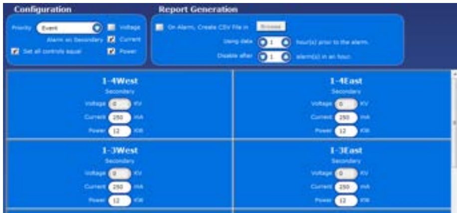
INDIVIDUAL T/R SET ALARMS CONFIGURATION
